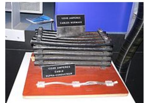
Electric cables for accelerators at CERN. Both the massive and slim cables are rated for 12,500 A. *Top*: regular cables for LEP; *bottom*: superconductor-based cables for the LHC
