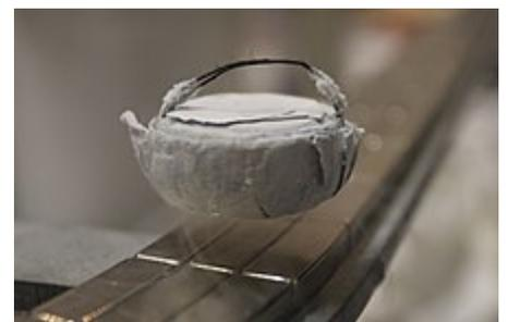
A high-temperature superconductor levitating above a magnet
